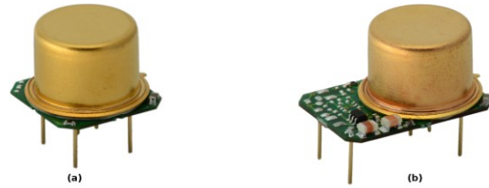
Figure 4. (a) the DIP8 compatible OCXO design (15x15x10mm or 15x15x8.5mm); (b) the DIP14 compatible OCXO design (15x20x10mm or 15x20x8.5mm).
