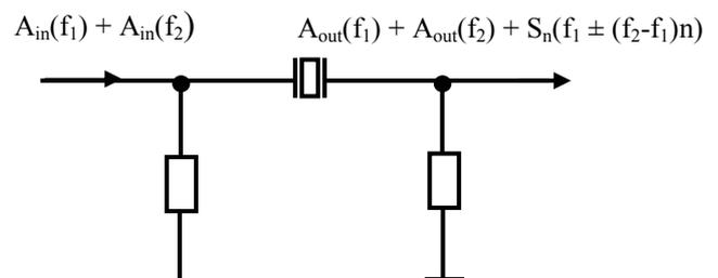
Fig.1. Schematic drawing of the simplest quartz filter.
