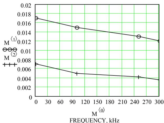
Fig. 5. Dependence of non-linearity coefficients  $N_r$  (corresponds to  $M^{(1)}$ ),  $N_c$  (corresponds to  $M^{(2)}$ ) on the electrode mass removing at initial mass-loading of 1 MHz.
